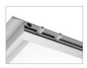
**NEBULA** fits perfectly on the kitchen cabinets, with sides **18mm** and **19mm** thick, thanks to the lateral pins. The configuration of the pins - quantity and position - can be customized thanks to the sliding guide that holds them.
